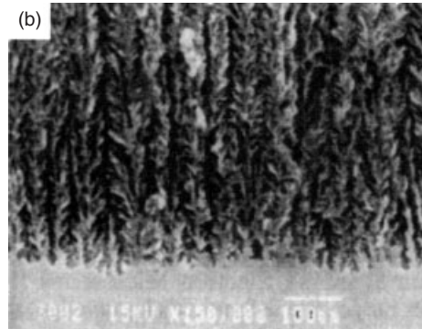
Fig. 10 TEM cross-sectional image of mesoporous structure formed by anodizing low-doped p -type Si (64% porosity) (from Ref. 89).
