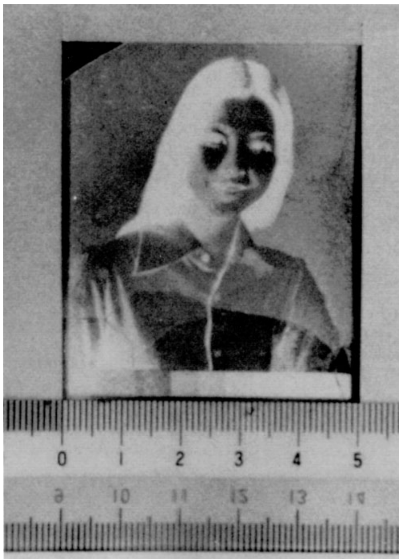
Fig. 1 Image recorded by using photoinduced deposition of metallic oxides on n -type semiconductor electrodes. This example shows \text{Ti}_2\text{O}_3 deposition on \text{ZnO} electrode from an aqueous solution containing a \text{Tl(I)} salt [12]. (With permission by the Electrochemical Society, Inc.)
