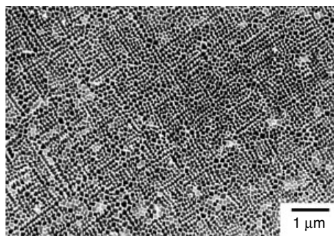
Fig. 9 SEM photograph of single crystal rutile \text{TiO}_2 surface ((001) face) after photoetching at +1.0 V versus SCE.
