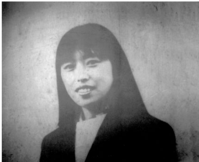
Fig. 2 Photoimage formed on a composite film of polyaniline and dispersed \text{TiO}_2 particles by projecting the positive image on the film that was immersed in 0.5 \text{ mol dm}^{-3} phosphate buffer (pH 7) containing 20 wt% methanol. The illumination was carried out with a 55 Xe lamp for 1 minute [49]. (With permission by the Royal Society of Chemistry).
