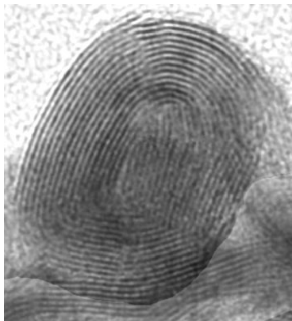
Fig. 7 TEM micrograph of NbS 2 nanoparticle with nested ("onion") fullerene-like structure (courtesy of Dr. M. Homyonfer, Weizmann Institute). The layer to layer distance is 0.59 nm.
